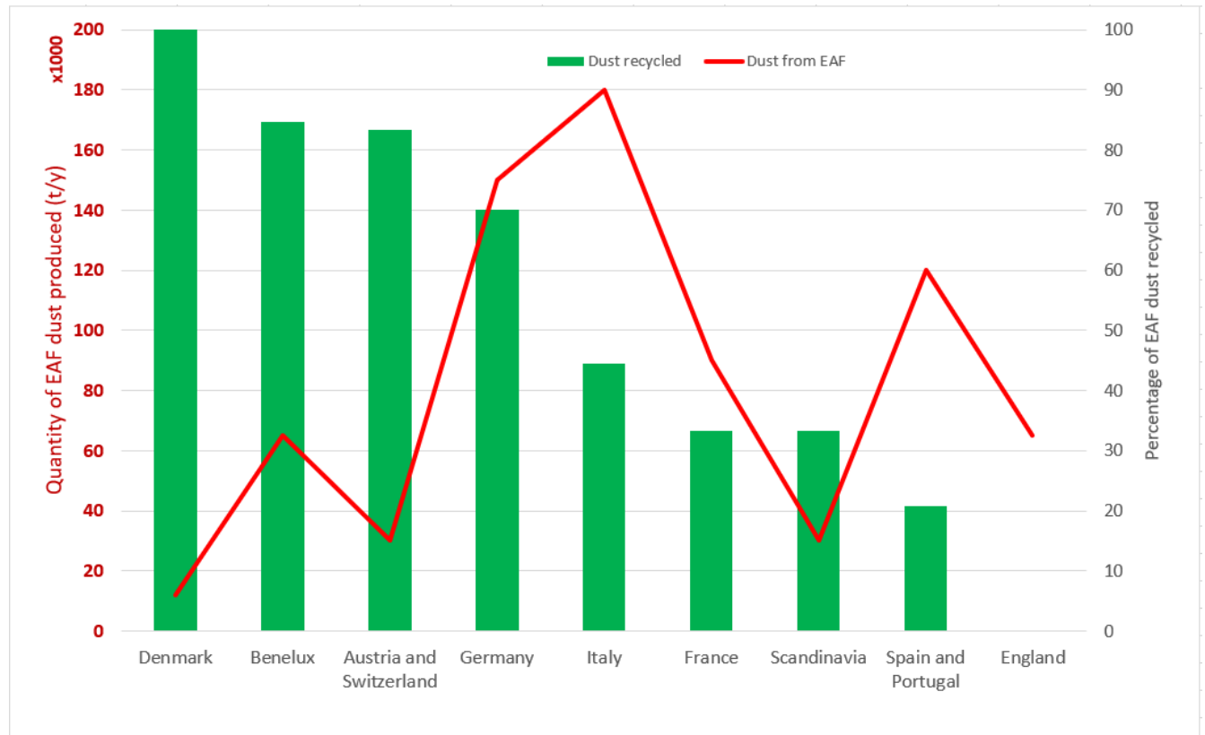
Figure 6. Situation of EAF dust recycling in the early 2000s
